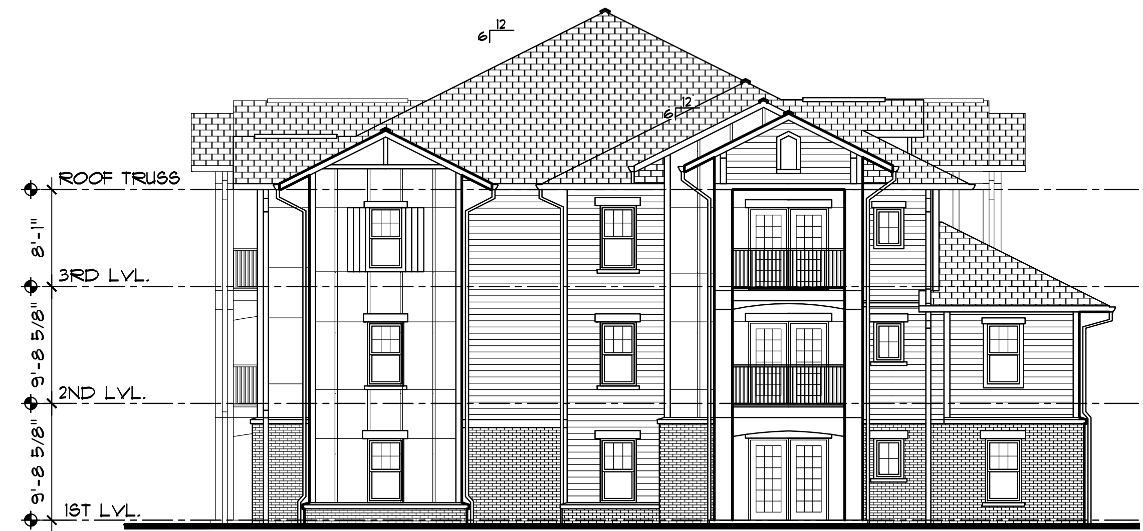
2 BLDG 200 SIDE ELEVATION 1/8" = 1'-0"
