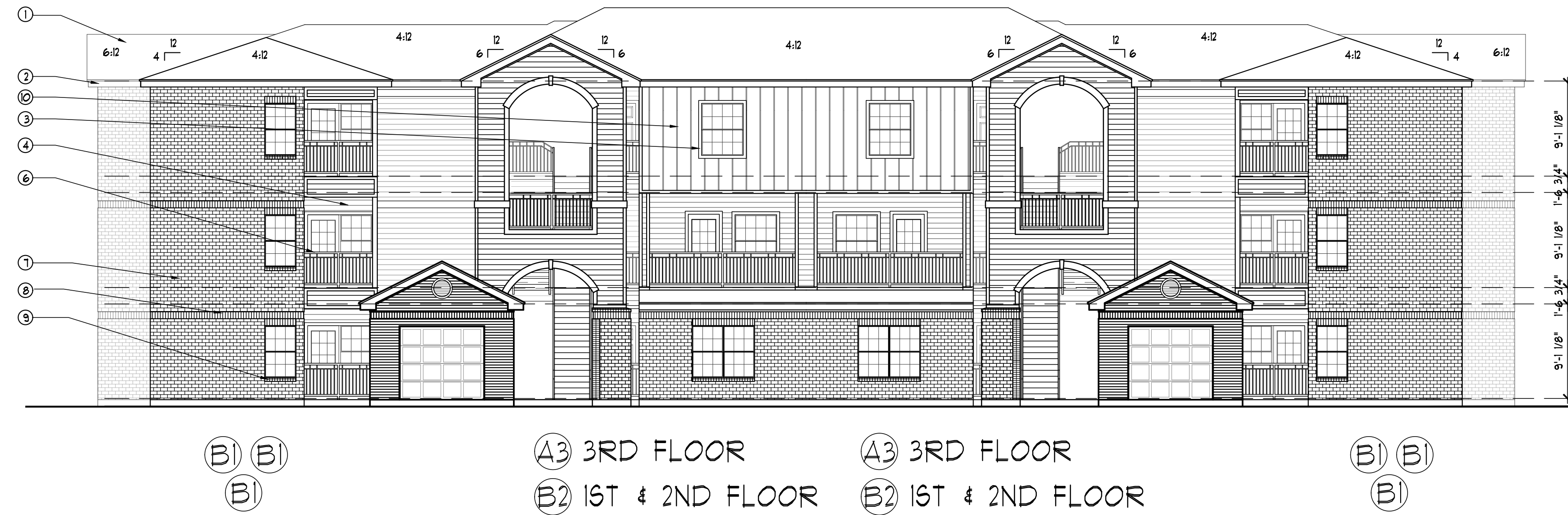
1 | BUILDING TYPE 2: BACK EXTERIOR ELEVATIONS 1/8" = 1' - 0"
