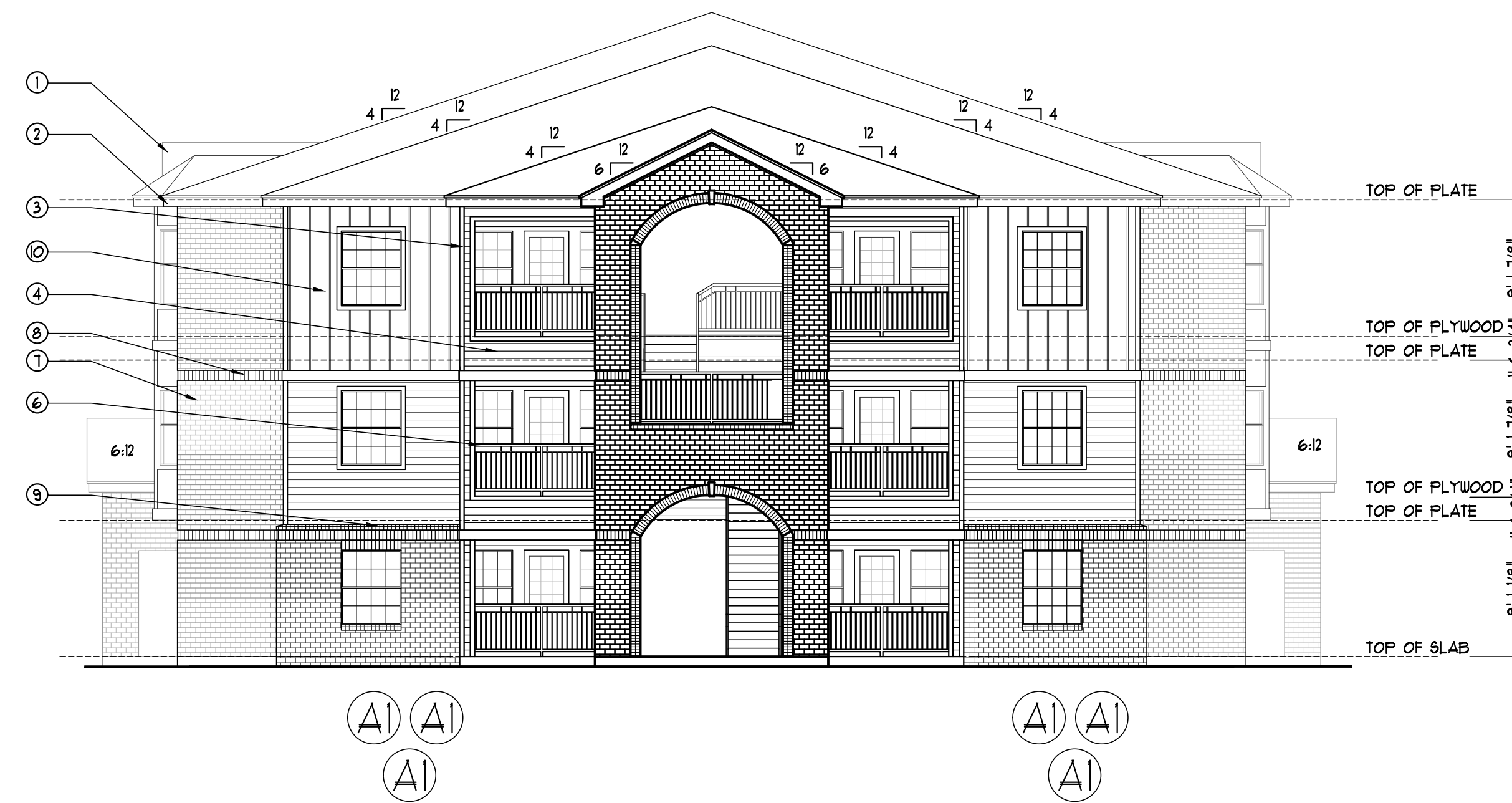
02 | BLDG. TYPE 4, EXTERIOR ELEVATION - SIDE 1/8" = 1'-0"
