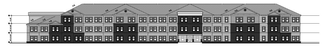
TOTAL EXTERIOR COMPOSITION (OPENINGS INCLUDED) = 9445 SQ.FT OF MATERIAL (BELOW SOFFIT) BRICK VENEER = 39%
