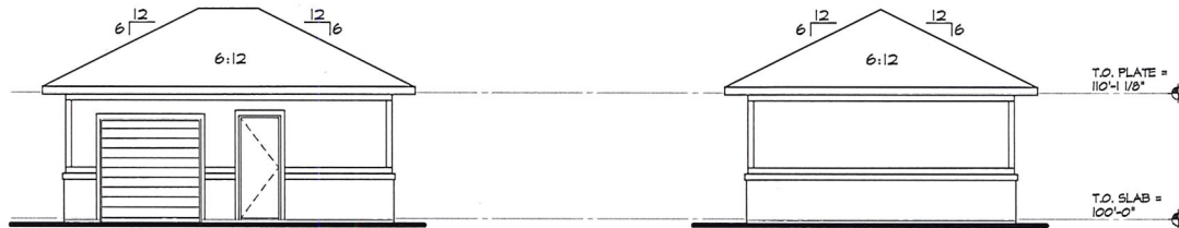
03 FRONT ELEV MAINTENANCE BUILDING SCALE: 1/16"=1'-0"
